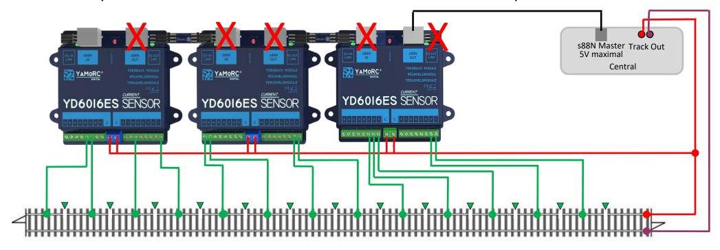
Maximum expansion: 96 feedback modules, consisting of five feedback modules with 16 inputs each in the entire "ES-Link" string.
