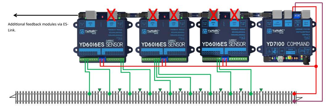
Maximum expansion: 96 feedback modules, consisting of five feedback modules with 16 inputs each in the entire "ES-Link" string.
