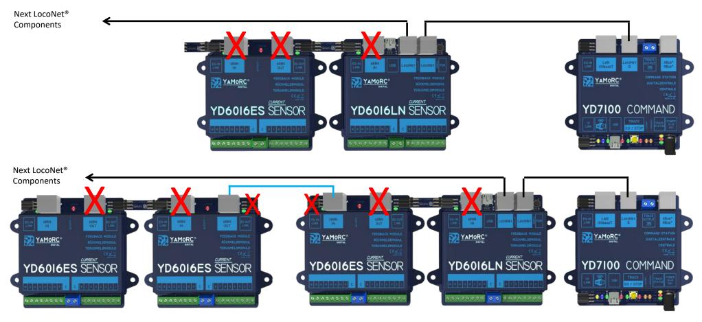
Maximum extension: 96 feedbacks, consisting of five feedback modules with 16 inputs each in the entire "ES-Link" line.
